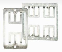
Mounting a flush mount wall plate without a back box is easy. Brackets insert into wall opening, flexible tabs bend up to secure the bracket to the opening. Standard screw holes accept all wall plate configurations.
